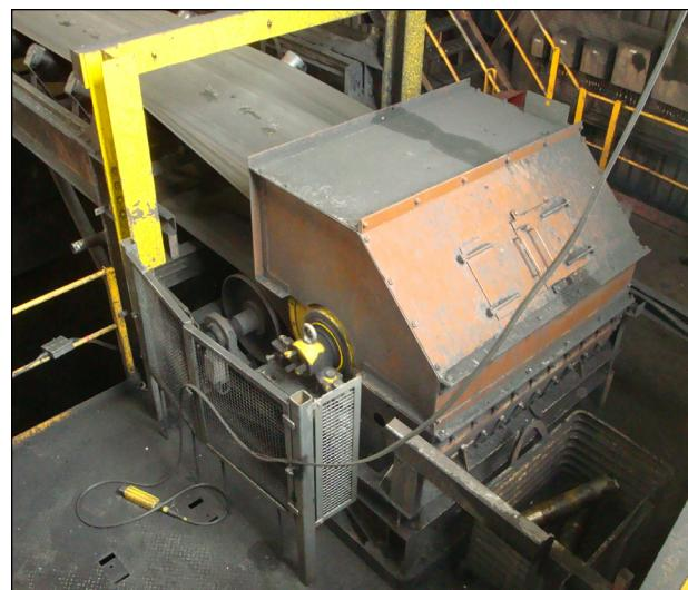
Model 800HD Rulmeca Motorized Pulleys drive bunker feed conveyors in Hunterston's train loading station. Each drive features a 100 HP 4 pole motor and three stage gearbox providing a 600 fpm belt speed.
