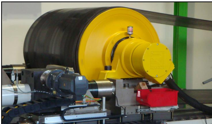
*Hunterston's 330HP 600 fpm model 1000HD under full load testing at Rulmeca facility in Germany, July 2011. 1000HD has a small footprint of 40.16" diameter x 59.06". Four mounting bolts simplify installation.*
